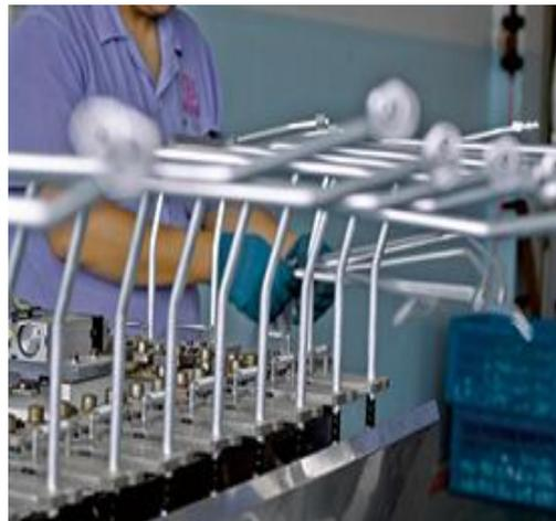
· 数控三层模自动弯管机 CNC automatic triple-layer bending machine
